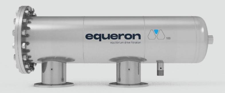
Introducing our technology-leading self-cleaning screen filters: Equeron Equilibrium Drive Filtration<sup>™</sup>. The hydraulicly balanced Equilibrium Drive<sup>™</sup> system rotates the suction nozzles across the screen in both directions without resistance. The mechanism does not require an electric motor or hydraulic piston.
