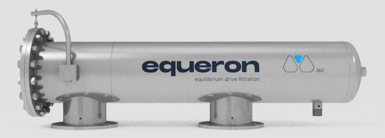
Introducing our technology-leading self-cleaning screen filters: Equeron Equilibrium Drive Filtration™. The hydraulicly balanced Equilibrium Drive™ system rotates the suction nozzles across the screen in both directions without resistance. The mechanism does not require an electric motor or hydraulic piston.
